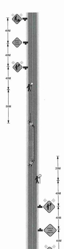
SPEED LIMIT ON CHADSEY ROAD IS 50KM PER HOUR ALL SIGNS WILL BE PLACED ON TRIPOD STANDS MTH FLAGS
